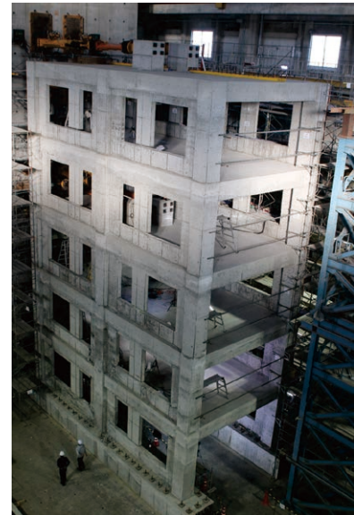
Resiliency of five story buildings tested at Building Research Institute (Tsukuba)
