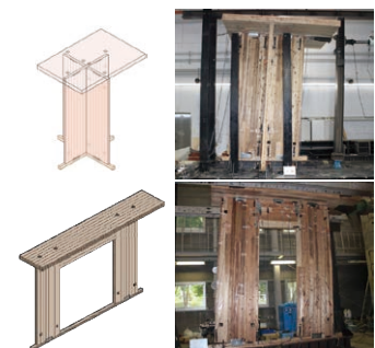
Full-scale lateral force test of shear walls by CLT panel construction
