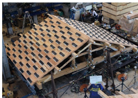
Full-scale lateral force test of a traditional gable roof frame
