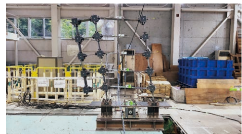
Shake-table test on the seismic ratcheting response of buildings with overhangs
