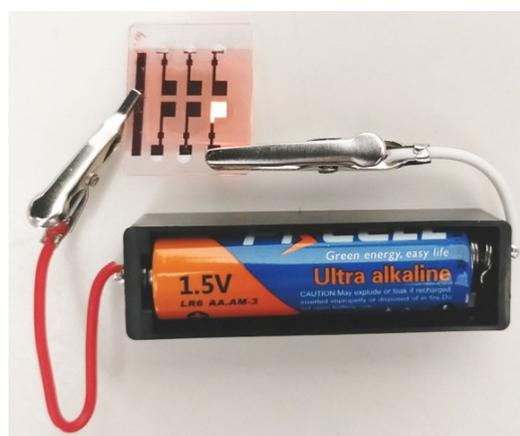
Organic light-emitting diode is operated by a 1.5 V battery.
