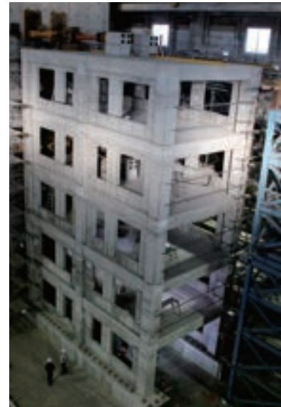
Resilience of five story buildings tested at Building Research Institute (Tsukuba)
